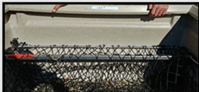
7. Lift one leg of the U-rod out of the feeder through the wide notch in the top rim and place the end of the other leg back through its mounting hole.
