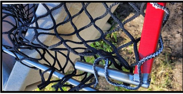
8. Place the slide arm back on the end of the U-rod. Feed the left side first to get the bar evenly on the rod, then feed the right side through the oval on the right end of the slide arm. Push the slide arm to the bottom of the U-Rod to be ready for installation back in the feeder.
