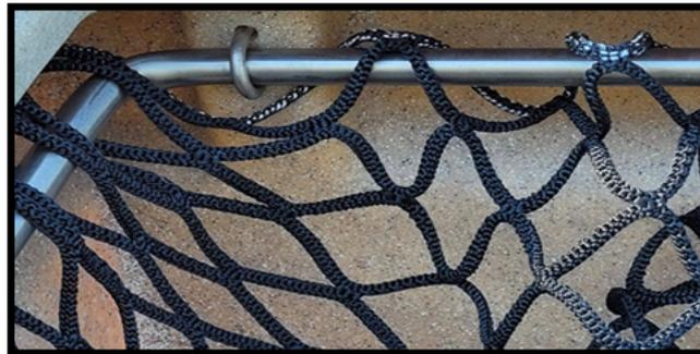
4. Recombine one of the U-bolts close to one set of alignment marks on the U-rod. Be sure not to entangle the net in the U-bolt.
